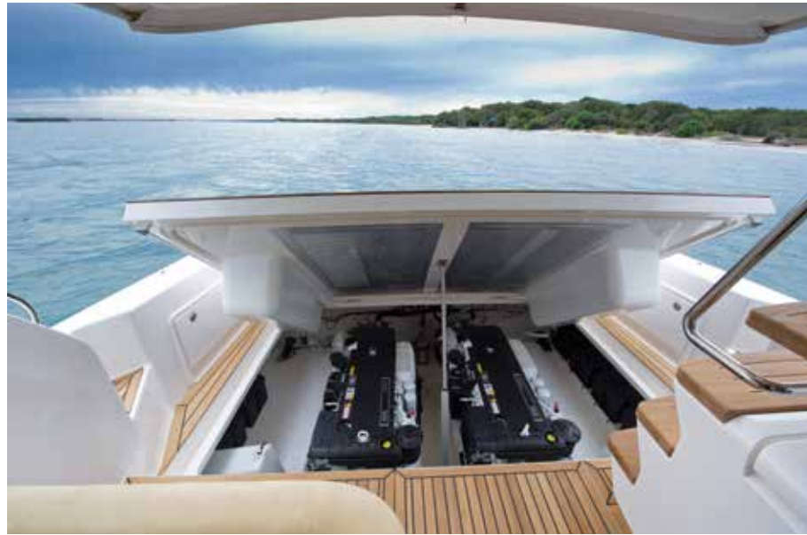
The 'floating' cockpit sole lifts to provide all-around access to engines.
